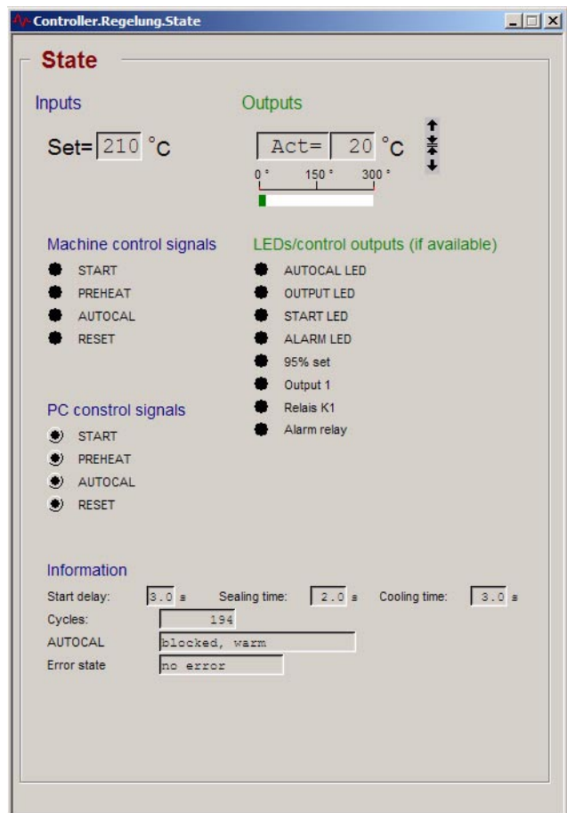
Example: "State" window on RES-445 controller, SW revision 101
